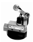
Enclosed Switches Series V6: Top Roller Arm Actuator, Adjustable with Steel Roller; 1NC 1NO SPDT Snap Action; 0.5 in - 14NPT conduit
